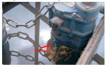
In the event of abrasive and corrosive utilization, stronger wear and tear will take place naturally in certain components. With regards to the above application wear and tear can take place mainly in impeller, suction plate, shaft sleeve, oil ring, mechanical seal and pump casing. Depending on the working conditions the lifetime of those parts might vary significantly and can be shorter than the legal warranty period.
